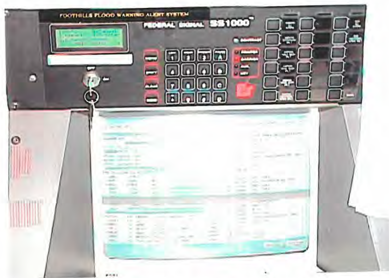
Siren system is activated by the buttons on top of the monitor.
