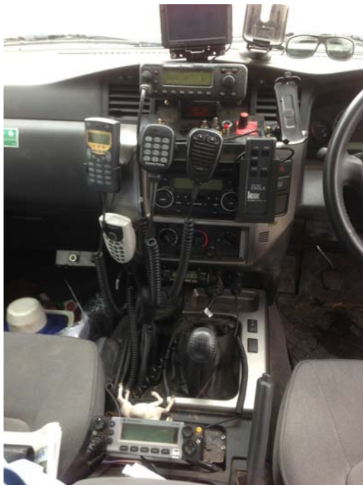
Figure 24 Radio communications available in Victoria Police's Swifts Creek based four wheel drive response vehicle, including VHF, HF and UHF options.
