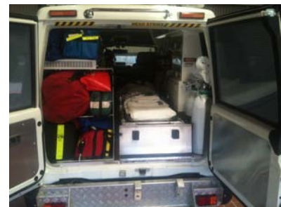
Figure 9: Ambulance Victoria's existing 4wd Toyota Land cruiser configuration - A dedicated 4wd retrieval vehicle suitable for wilderness environments
