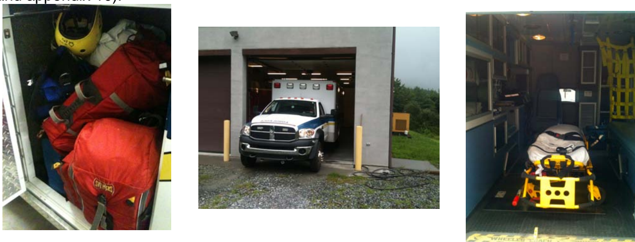
Figure 7: Burke County Special Operations vehicle. A RAM 4500 four wheel drive (centre). Patient compartment configuration is standard (right), while wilderness and vertical rescue equipment is stowed in a side locker (left).
