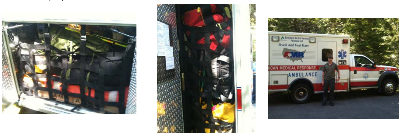
Figure 8: American Medical Response Portland Reach and Treat (RAT) team vehicle. A four wheel drive ambulance (right) with wilderness and vertical rescue equipment stowed in side lockers (left and centre).
